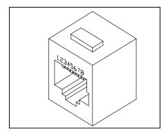
Figure 7: RJ-45 Receptacle
